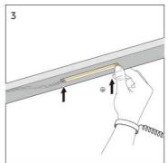
Clean the environment part to be attached with a cloth, as shown in Figure 1, and then tear off the 3M tape on the back of the light belt, and finally stick the light belt on the clean place.
