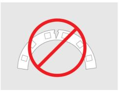
Do not bend the LED strip on a horizontal plane
