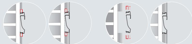
Fylo+ is fitted to be installed into plasterboard walls. To install it on already existing walls, simply remove the side wings included in the profile.
