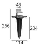
Sacchetto / Kit di fissaggio - PICCHETTO PER RUBBER + STAFFA PICCHETTO PER RUBBER + STAFFA PICCHETTO+STAFFA D114X204 per Rubber 3D, Rubber 3D Concrete, Rubber 3D 48V, Rubber 3D Optic, Rubber 3D Pixel
