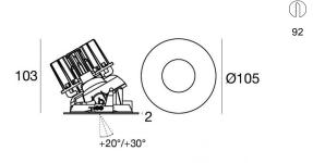
Max inclination: +20° with double panel +30° with single panel
