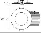
Finishing casing Die-cast Aluminium EN AB - 46100 Material Colour Processing Powder coating
