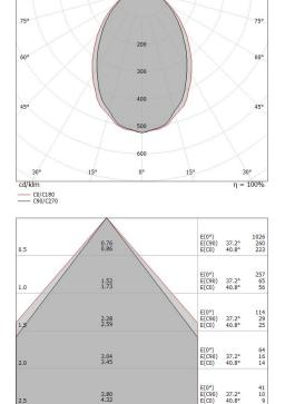
4.55 3.0 5.18 Distance [m] Cone diameter [m] — C0/C180 (Half-peak divergence: 81.6\*) — C09/C270 (Half-peak divergence: 74.4\*) E(0°) E(C90) E(C0)
