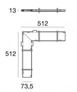
Finishing casing Material Aluminium 6060 Colour White Processing Powder coating
